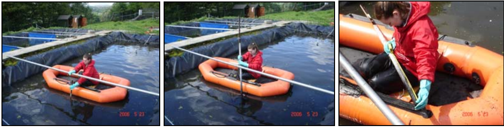
Figure 4.8: Measuring the sludge depth profile
