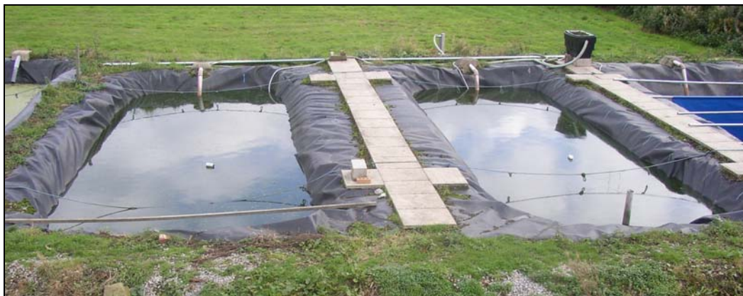
Figure 4.1: The two primary facultative WSP at Esholt WWTW used over the research period. The pond in the left of the picture is the Blue pond, and the pond in the right, the Green pond.
