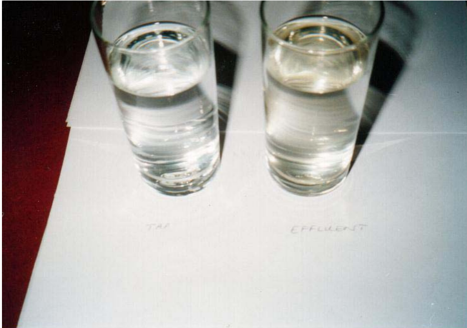
Plate 4-1. A typical effluent sample from system 1 compared to tap water.
