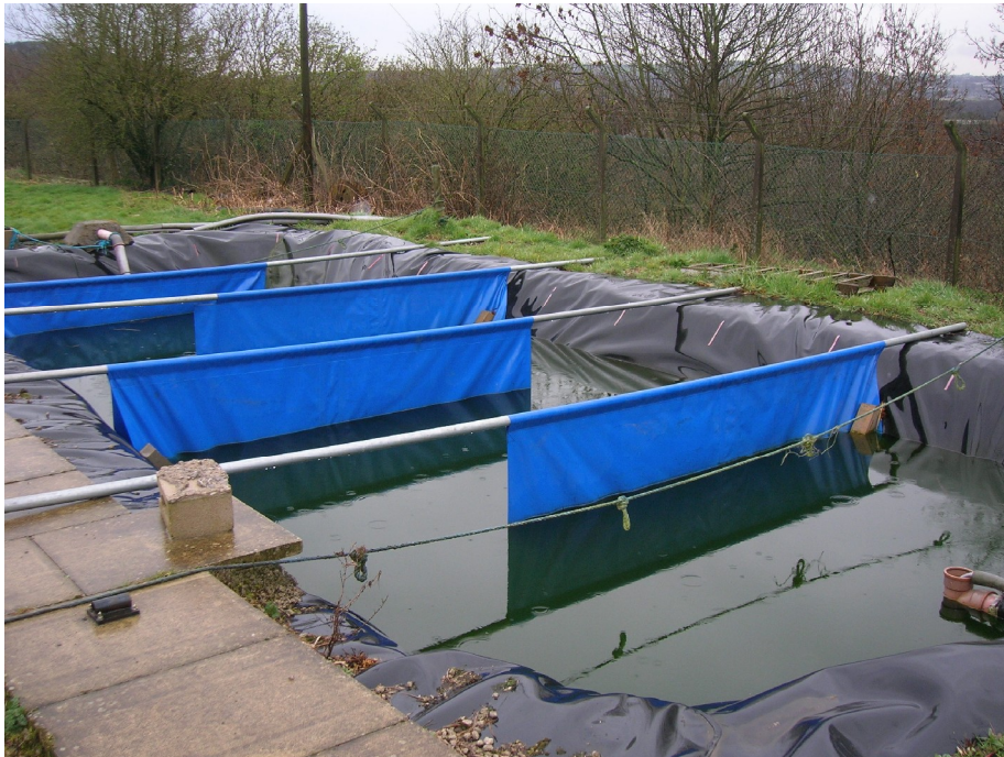
Figure 4.2 Layout of the four-baffle configuration in the pilot-scale pond
