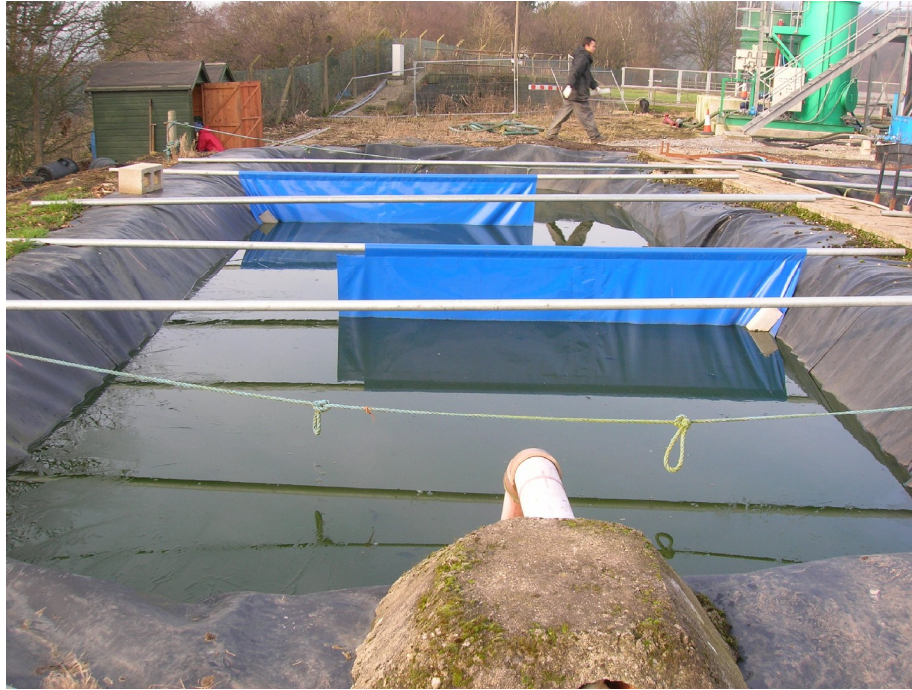
Figure 4.1 Layout of the two-baffle configuration in the pilot-scale pond
