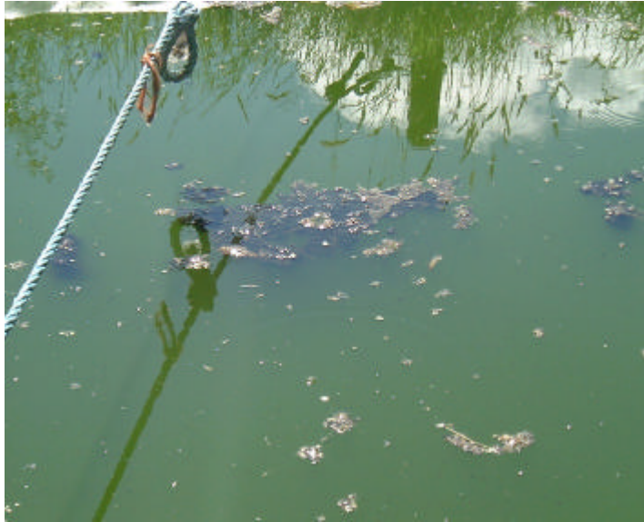
Figure 5.51 Sludge feedback bringing settled leaves back to the surface (summer 2002)
