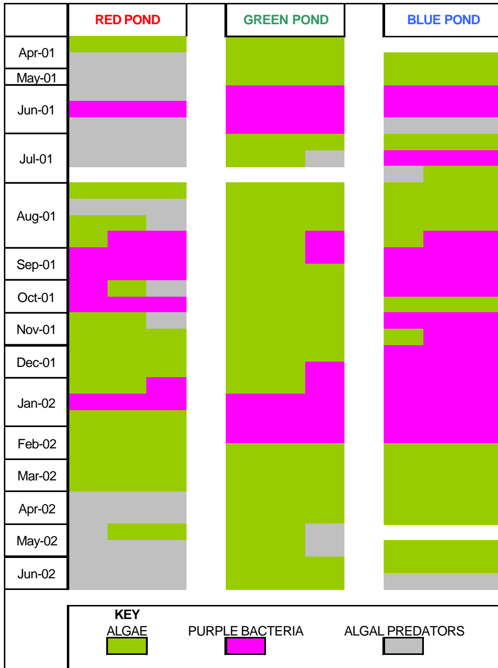
Figure 5.35 Dominant organisms found in the effluent samples from all ponds
