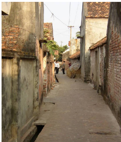
1. Lane in a small town near Hanoi, Vietnam (notice partially covered drain at left used for both greywater and stormwater)
