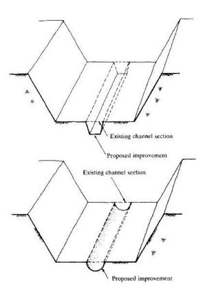
Figure 1. Stormwater drain modified to carry greywater flows (Kalbermatten et al., 1982).
