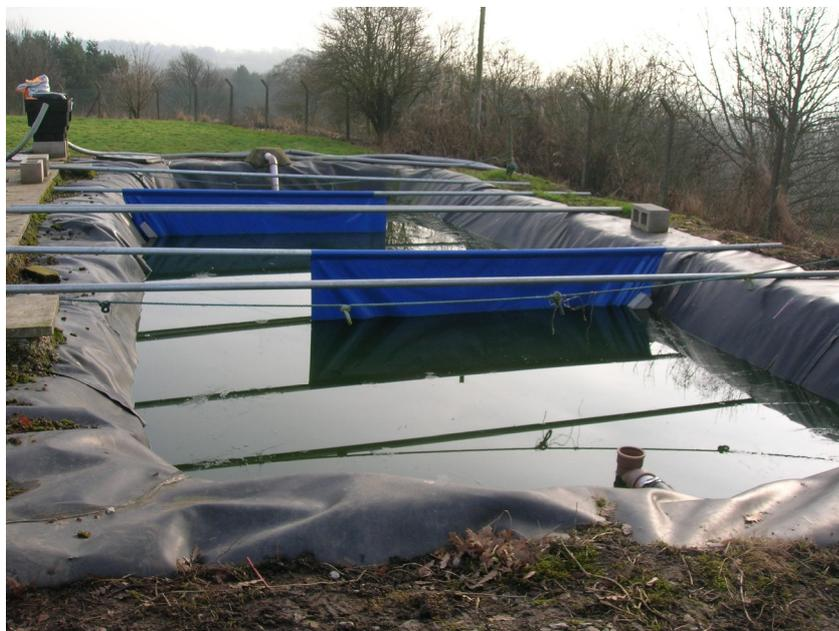
**Figure 1.** Plan view of the twin baffles in the pilot-scale primary facultative pond.
