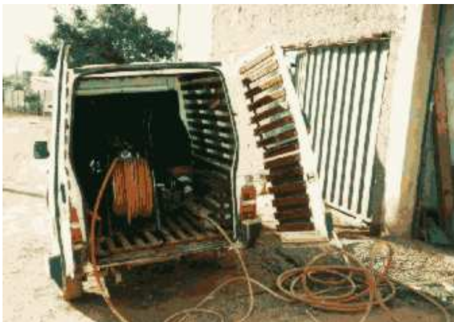
Figure 5.7 Vehicle-mounted water-jet unit used for simplified sewer O&M in Brasília.
