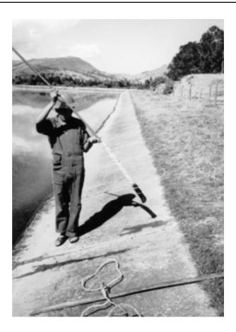
**Figure 7.2** The "white towel" test for measuring sludge depth.
