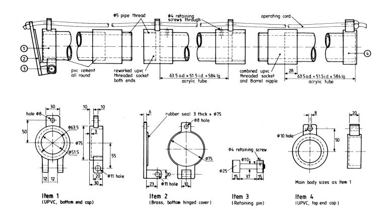
**Figure 7.1** Details of pond column sampler. The overall length (here 1.7 m) may be altered as required. The design shown here is a three-piece unit for ease of transportation, but this feature may be omitted. Alternative materials may be used (for example, PVC drainage pipe).
