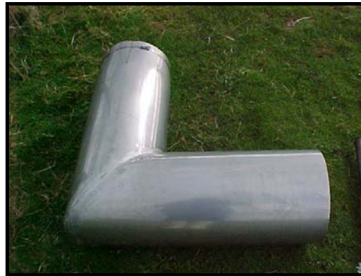
Figure 9-3 Inlet insert used in field trial
