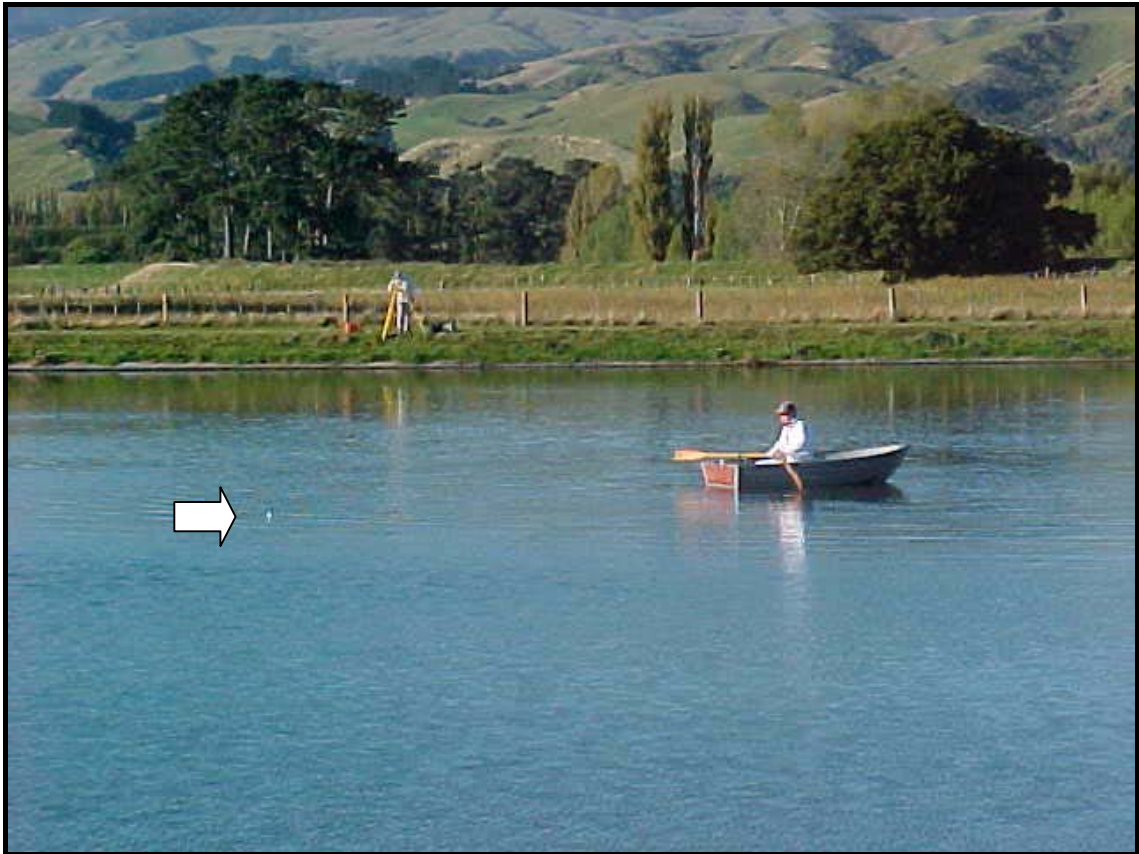
Figure 10-2 An alternative to tracer studies is ‘drogue tracking’. The arrow shows the surface indicator of an underwater drogue.
