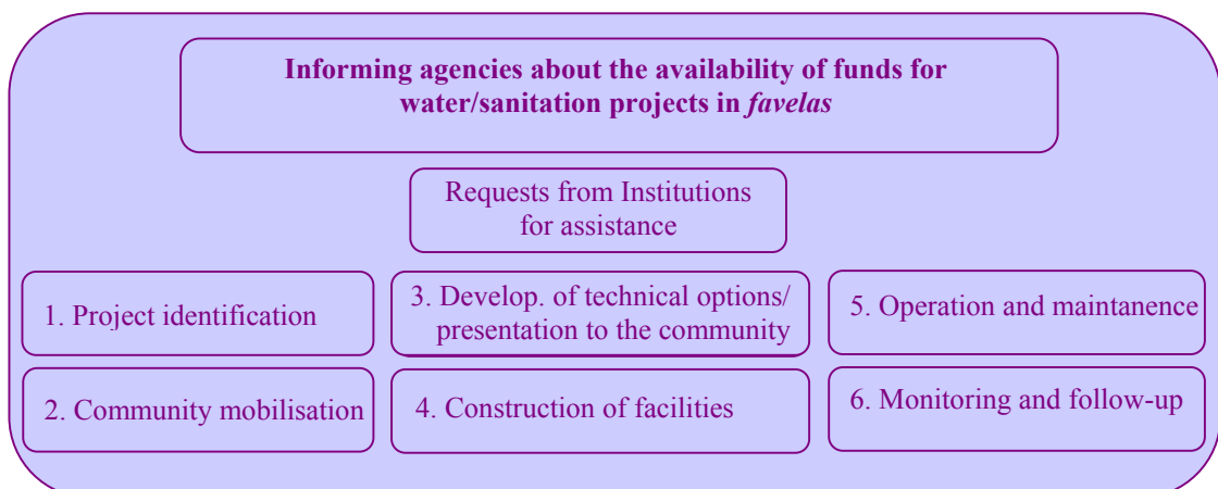
Figure 2.10 - Model for the implementation of PROSANEAR I projects. Based on Katakura & Bakalian, 1998.
