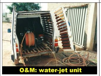
Operation and maintenance of the simplified sewer network in Brasília is done with a water-jet unit mounted in a commercial van. If there is a blockage in the sewer, then a high-velocity water jet is introduced at the junction box just upstream of the blockage, and the blockage is then jetted down the sewer to the next junction box where it is caught and removed.
