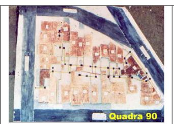
This slide shows the layout of Housing Block 90 and the initial thoughts on where the simplified sewers would be positioned. These are shown as yellow lines and the black squares are junction boxes.
