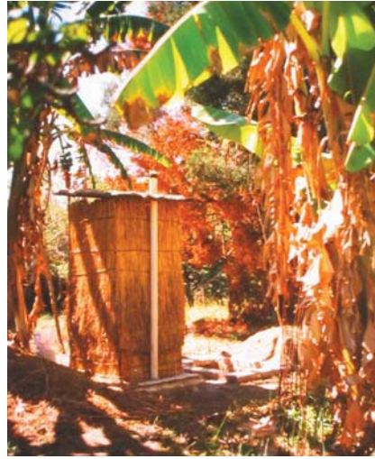
Figure 4-16: Fossa alterna with grass walls
