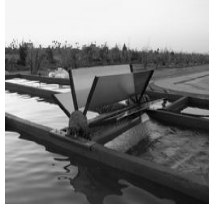
Figure 3 : The paddle wheel in operation
