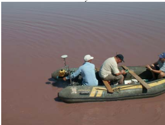
Fig 3. Echo sounding at El Jem: system configuration. The GPS antenna is clearly visible
