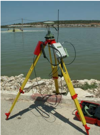
Fig 1. Reference station: calculation of error and link by radio modem
