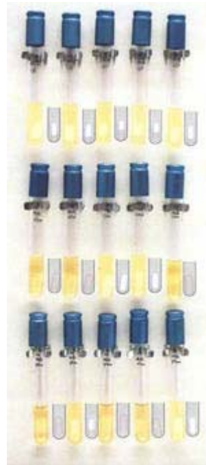
Fig. 16. After incubation at 44°C for 24 h, five of the tubes containing 1 ml of sample are positive (gas production), two of those containing 0.1 ml (1 ml of the 1:10 dilution), and two of those containing 0.01 ml (1 ml of the 1:100 dilution). For clarity, accompanying schematic drawings show positive and negative tubes. From Table 3, the MPN is 950 faecal coliforms per 100 ml of sample (treated wastewater).
