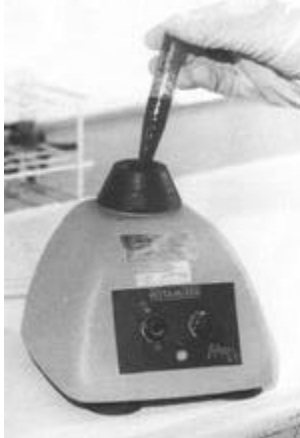
Fig. 5a. Homogenization of the sample can be carried out with a vortex mixer.
