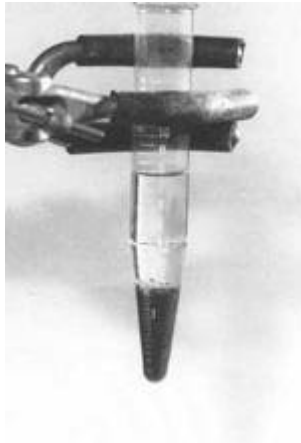
Fig. 4. The pellet with 1 volume of buffer and 2 volumes of solvent.
