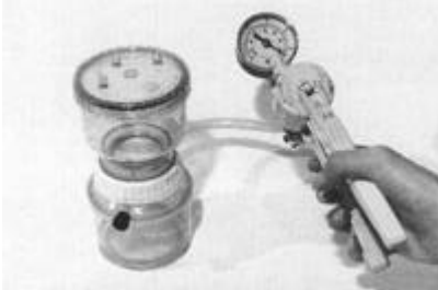
Fig. 21. Using a manual vacuum pump to filter the sample through the membrane filter.
