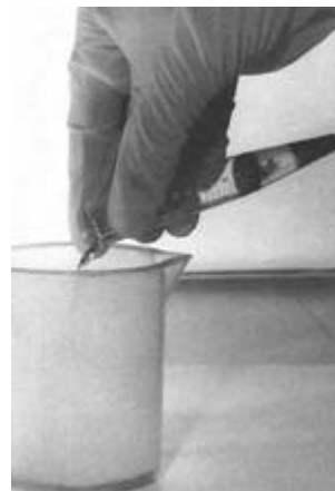
Fig. 5b. The sample can also be homogenized by hand.
