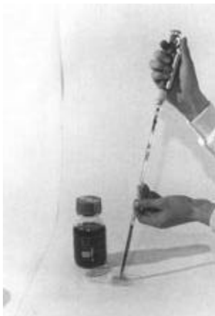
Fig. 17. Adding 1.8 ml of sterile membrane lauryl sulfate broth to a Petri dish containing a sterile absorbent pad.
