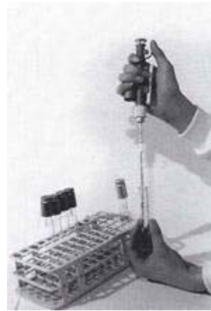
Fig. 14. Adding 1 ml of the 1:10 dilution to a test-tube containing 5 ml of medium A-1 and an inverted Durham tube.
