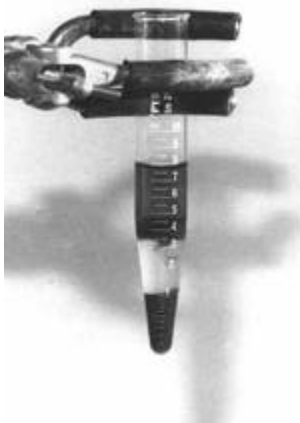
Fig. 6. Separation of the sample into three distinct phases after centrifugation.
